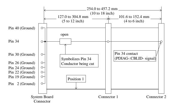
Figure 3.11 Cable configuration
